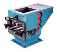
The Magnet's redesigned housing has been engineered to provide superior strength to bear the weight of infeed hoppers and other processing components. We grind the inside of the housing smooth to facilitate cleaning and prevent powdered colorants and resins from clinging to the interior surfaces. The unit also features a slide gate that is completely enclosed within the housing so that any powders that cling to the slide gate will be redirected back into the product flow.
