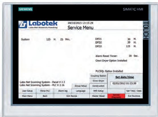
Full service menu with timers and complete alarm log
