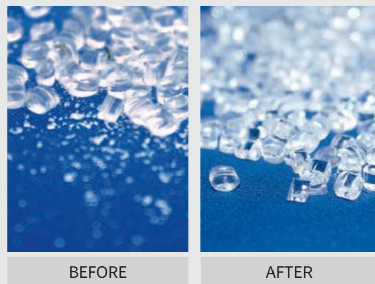
PMMA raw granulate before and after dedusting.
