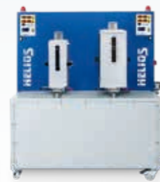
HELIO®MAT 6/12 for drying containers 6 or 12 liters
